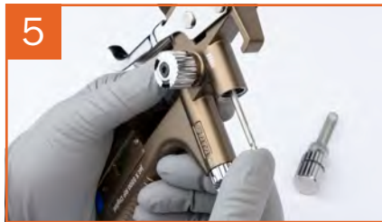
5 Assembly of the paint needle
