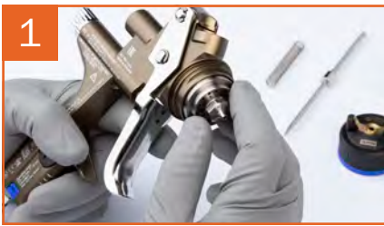
1 Assembly of the fluid tip
