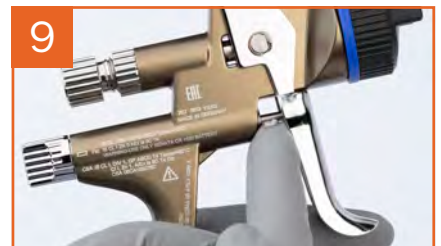
9 Lubricate visible area of air piston rod
