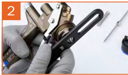
2 Hand-tighten fluid tip with universal spanner
