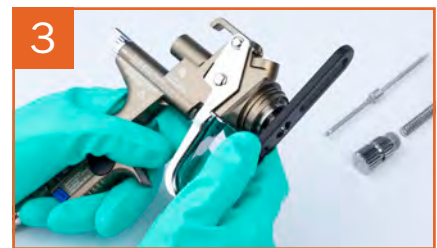
Unscrewing the fluid tip with the ring spanner integrated in the universal spanner.
